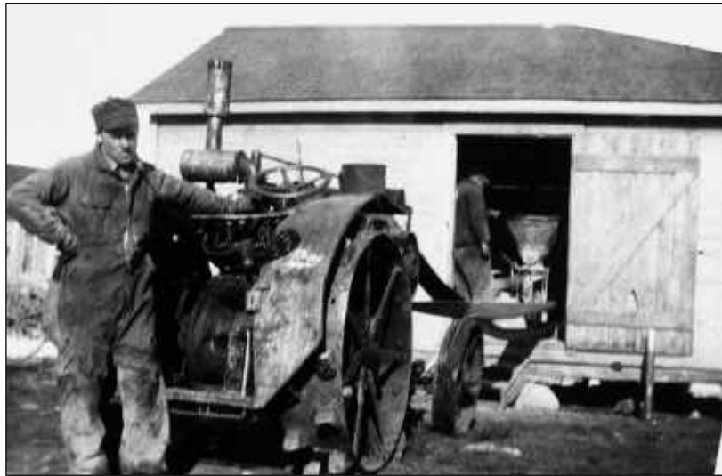
Above: Frank and Louis Osioway using the Oil-pull Rumsley's Tractor to power the feed mill on the Mike Osioway homestead, Wheathill S.D. , c1940. FL-167.
