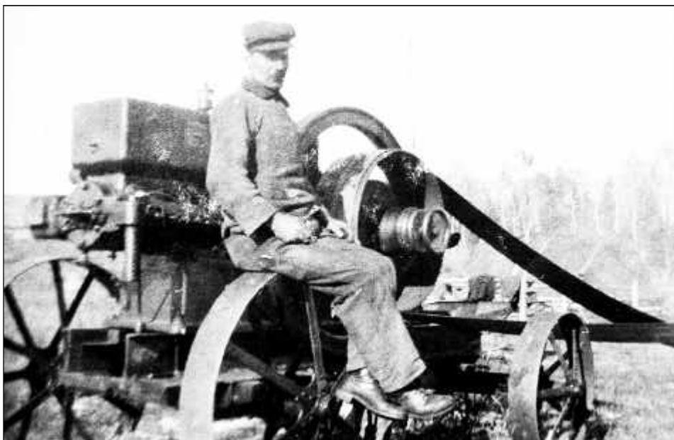
Above: During the early decades a few horse-drawn 'stationary-engines' such as the one depicted above powered threshing machines and saw mills in the district. The self propelled Case steam-engine was more versatile but more expensive to purchase. RTM-033.
