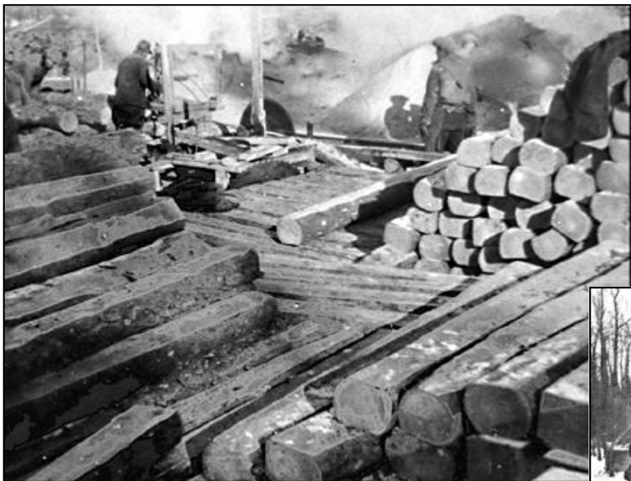
Left: Cutting railway ties at Davis' sawmill at Mantagao Lake area northwest of Fisher Branch, 1941. A tremendous railway expansion was taking place in Western Canada when our pioneers began arriving. With this, there was a great demand for ties. Once the rail tracks came to Arbrog (1910) and through Poplarfield (1914) local people were able to tap the large stands of tamarack growing on the low lands, and this became the first large-scale marketable product from their communities. In the later years the local loggers continued to supply ties as part of their mill operations. WT-001.
