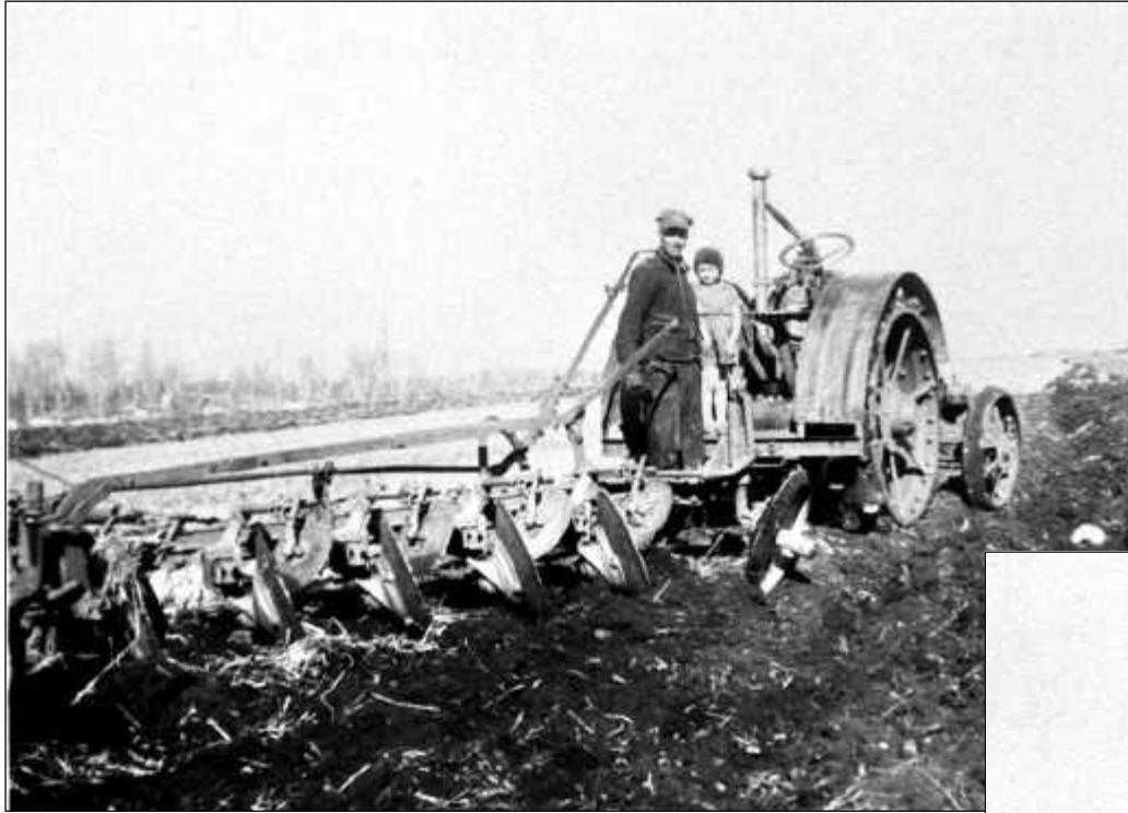
Left: Mike Marko and five year old niece, Bernice, pose for a quick photograph during a break in plowing, c1942. Mr. Marko is pulling a 5-bottom disc plow. These plows were heavily constructed and without hydraulics, it required a strong operator to lift the discs on turns. This piece of machinery was more commonly known as a "one-way", as it was almost impossible to back up. Note also, the full quarter section depth of open field in the distance. Beginning in the late 1920s, the large marshes located between the Hamrlik and Zbaraz districts began to be drained, giving rise to some excellent, largely stone-free, cropland. FL-024.
