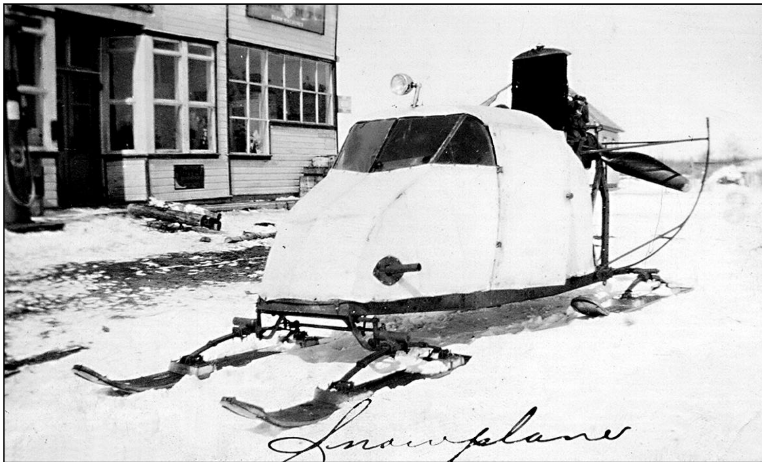
Above: The only known photo of the 'snow-plane' constructed by Mike Torbiak during the early 1940s. Its propeller and airplane engine, it could be heard for miles when it was out travelling the countryside. In an unfortunate accident, Peter Torbiak Sr. was seriously injured when he was struck on the chin by the spinning propeller. RTM-046.
