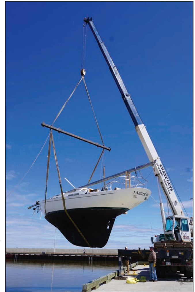
Above: Spring launching of the sailboat Aegir III, owned by Bruce Harmer. This beautiful Alberg 37 weighs 7250 kilograms and, along with several others, requires a large mobile crane for launching. In recent years larger sailboats have become more common in the Gimli Harbour.
