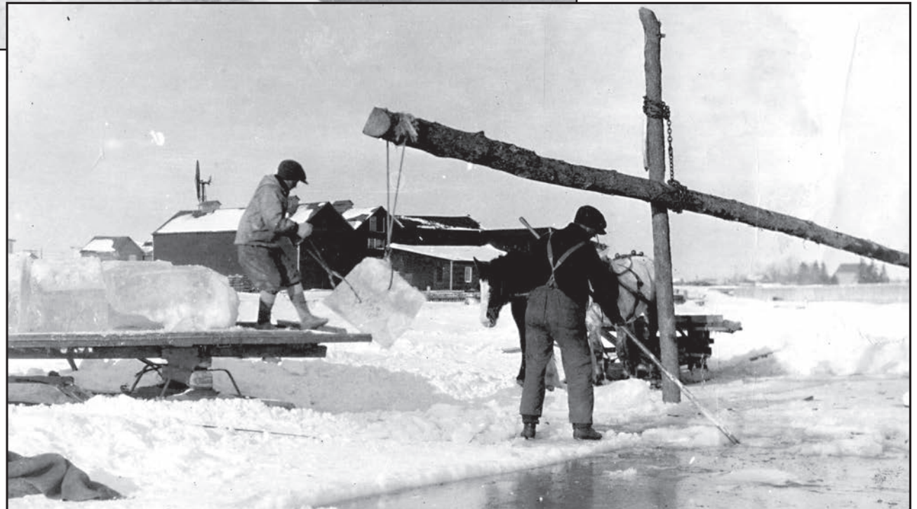
In late winter, in the time before modern refrigeration, the lake provided the tools for keeping fish from spoiling. Using large hand saws and a primitive log hoist, large blocks of ice were removed from the lake and hauled by horse-drawn sled to an ice storage building in the Gimli harbour. (NIHM Photos.)
