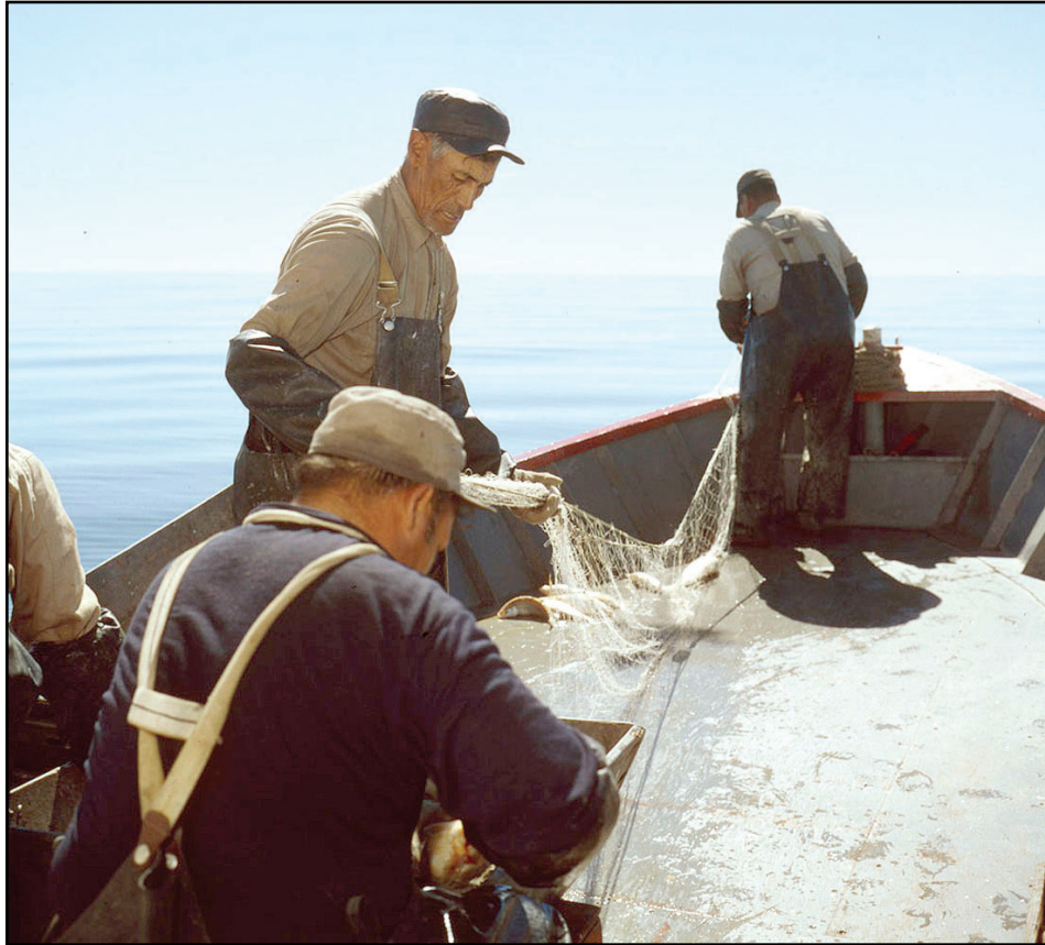
Above & Right: Photographs taken by Canada Department of Fisheries staff during an inspection visit in 1961. Fishermen tending their nets on a rare calm day on the lake. Labour-saving nylon nets have replaced cotton and linen ones that had to be pulled from the lake every few days and dried. ( L&AC Website. )
